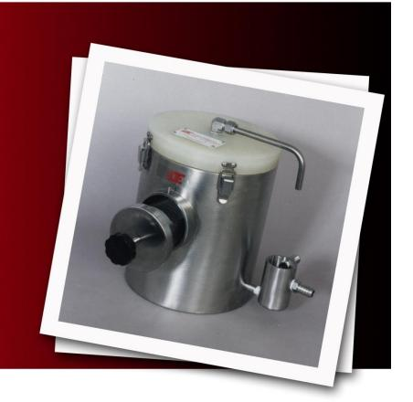
The Pulp Brightness Reversion Apparatus consists of a stainless steel vessel that holds thirty-two 25 cm<sup>2</sup> pulp specimens. The insulated vessel is heated with an external hot plate (not supplied). An internal drip roof prevents any condensation from falling onto the samples.
