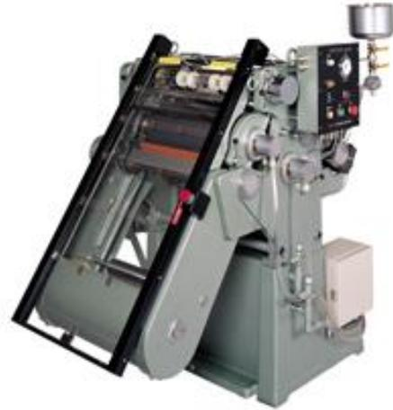
As an option, there is a model equipped with a coating-liquid heating and circulating system and with a device to humidify the press roll.
