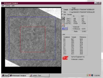
The Watermark Quality Analysis Software display after the sample has been aligned with the Reference
