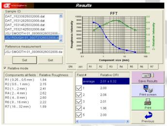
OpTiSurf results display of the FFT Roughness Intensity (blue curve) and the Relative Roughness Intensity (green curve) between a test sheet and a reference sheet
