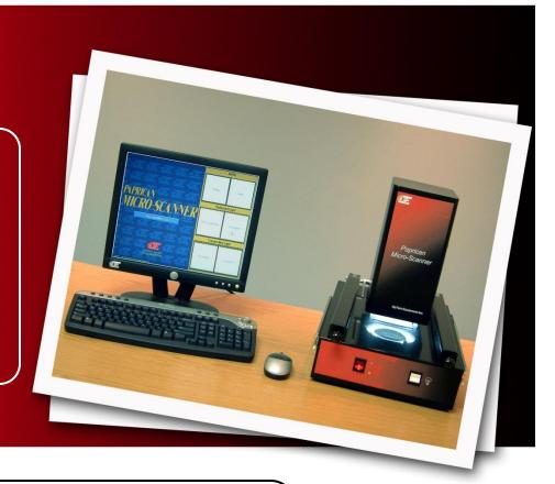
Camera based image analyzers have superior depth of field which easily accommodate rough or poorly formed sheets.
