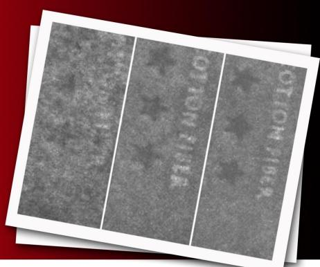
Watermarks are imaged in transmitted light with the PPF or Micro-scanner, and images stored. The stored Sample images are opened by the Watermark Image Analysis software. The Watermark Intensity Ratio and Sharpness Difference are then determined relative to a Reference image. The results include:
