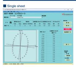
For single sheet measurements, A4 size is the standard sample size. Minimum is 15 x 15cm. The following main measurement results and TSI graphics are output. These can now also be output to Excel files. It is also possible to recall past data and compare it with current data on the same screen.
