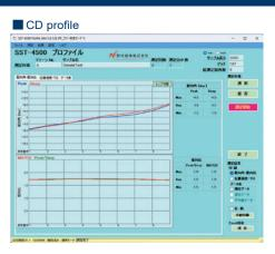
A long CD sample is automatically measured at specified intervals using the sample feeding device (optional), and profile data is output. It is also possible to output data measured in cut sheet mode on multiple cut samples taken along the CD, as well as automatically measured data on MD samples. It is also possible to compare with past data.
