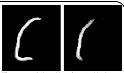
The same cellulose fiber viewed with circular polarized light (left) and linear polarized light (right). The ends of the curled fiber disappear in linear polarized light.
