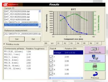
OpTiSurf results display of the FFT Roughness Intensity (blue curve) and the Relative Roughness Intensity (green curve) between a test sheet and a reference sheet
